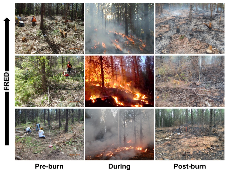
Figure 2. Sampling masticated fuels pre-burn (left), representative fire behavior ranging from low intensity (bottom row) to high intensity (top row) during prescribed fire experiments (middle), and post-fire fuelbed conditions (right). Fire intensity is indicated here as Fire Radiative Energy Density (FRED). Photos from Sparks et al. (2017).
