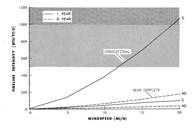
Figure 2.--Byram's fireline intensity for 1-and 5-year-old lodgepole pine fuels left after logging to conventional (C) and near-complete utilization standards (NC) at Union Pass. Shaded areas warn of unacceptable hazard. Table 1.--Rate of spread for post-logging Douglas-fir/larch slash 1 year and 5 years after cutting at 0, 5, 10, and 15 mi/h windspeed, Coram.
