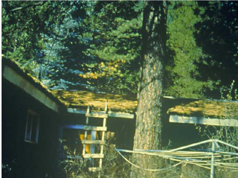
Figure 27 —One of the home photos that students assess in this activity. Note the presence of ladder fuel. Photo courtesy of Montana Department of Natural Resources and Conservation.
