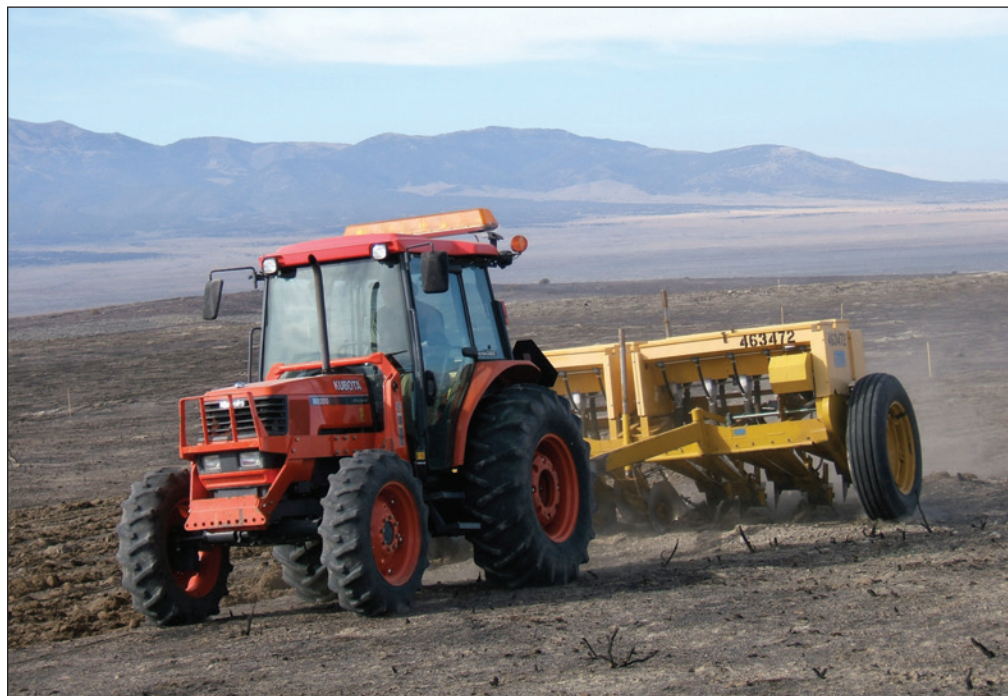
Figure 11 —A rangeland drill in use at the burned site of the Scooby Fire, in northern Utah, in 2008. This drill was modified for seeding diverse mixtures of native plant species. It is an example of the specialized seeding techniques under development for restoring sagebrush ecosystems following wildfire in the Great Basin (photo by Beth Newingham, USDA Agricultural Research Service).
