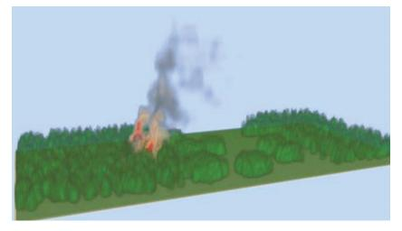
Figure 3.2. Physics-based fire models such as FIRETEC (pictured here) simulate fire spread in three dimensions and at much higher resolution than standard fire models. These detailed models are useful for exploring how disturbances, such as MPB outbreaks, affect fuel loads and fire behavior (figure by Russ Parsons, USDA Forest Service).
