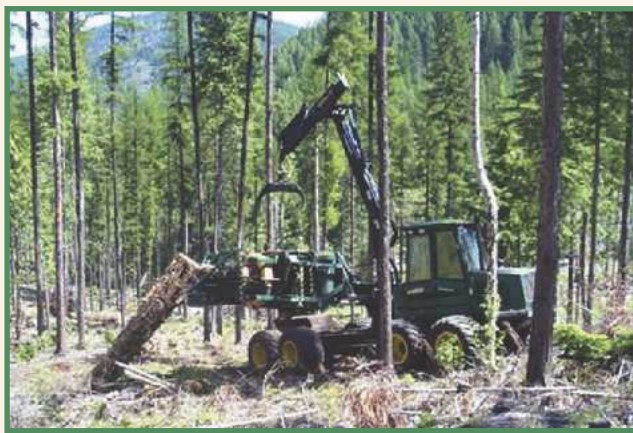
Figure 4. — Specially designed harvesting equipment bundles biomass into bales for bioenergy systems.
