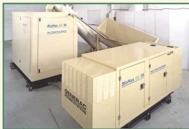
Figure 3. — This portable modular power system gasifies wood pellets or other biomass and generates 15kW electricity.
