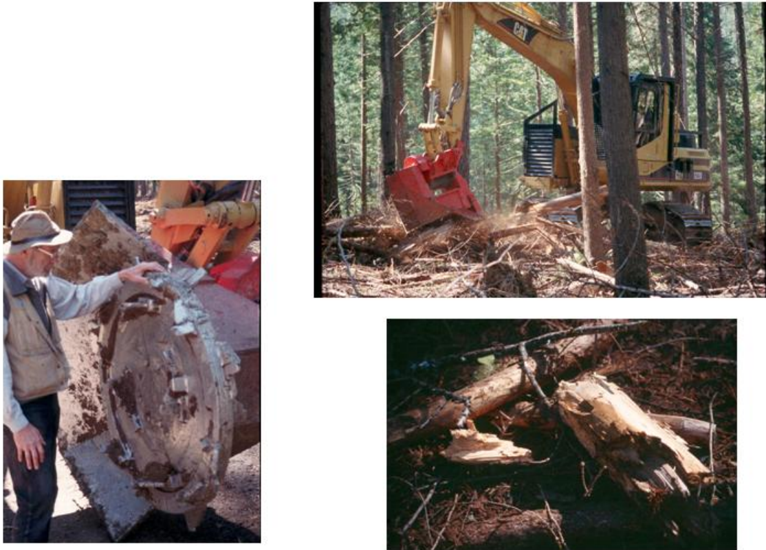
Figure 4. The machine we used to masticate the surface fuels had a horizontal rotating head that could articulate, reach 25 feet horizontally, and reach approximately 15 feet vertically.
