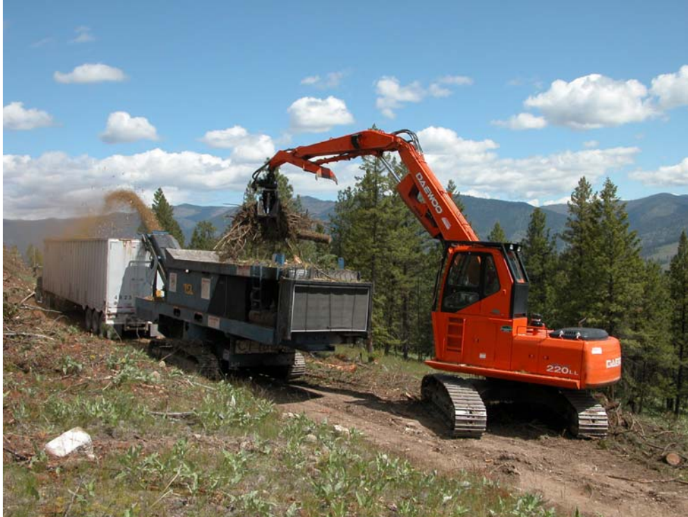
Figure 3. A Daewoo Model 220LL Log loader was used to load slash into the Universal Refiner grinder at the Dry Creek site.
