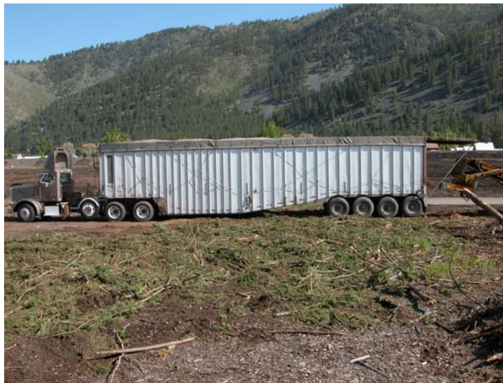
Figure 13. 148 cubic yard capacity chip vans were also used in the study. They could only haul about 34 tons (green) of product due to legal maximum weight restrictions.
