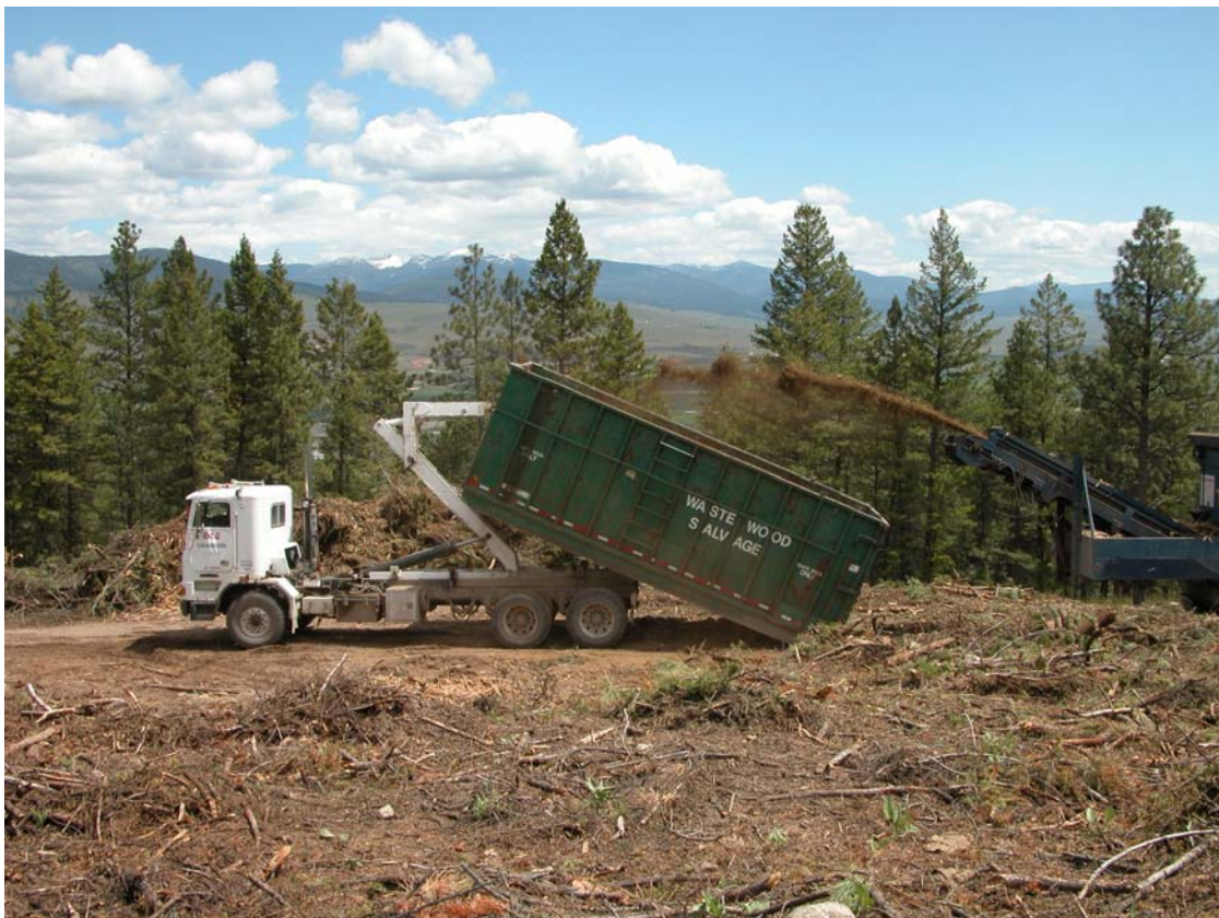
Figure 5. Loading tilted roll on/off container while on truck.
