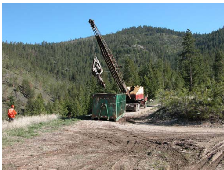
Figure 9. Loading roadside staged roll on/off container.
