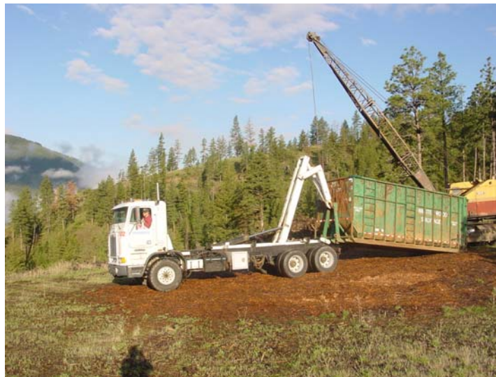
Figure 7. Loading roll on/off container for transport. The roll on/off container truck system used in the study was a cabover Freightliner tractor (430 hp) with a Stellar Industries hooklift conversion and a pup trailer. The roll on/off containers had a capacity of 48 cubic yards each. This system was leased from DCT Chambers of Vernon, British Columbia.
