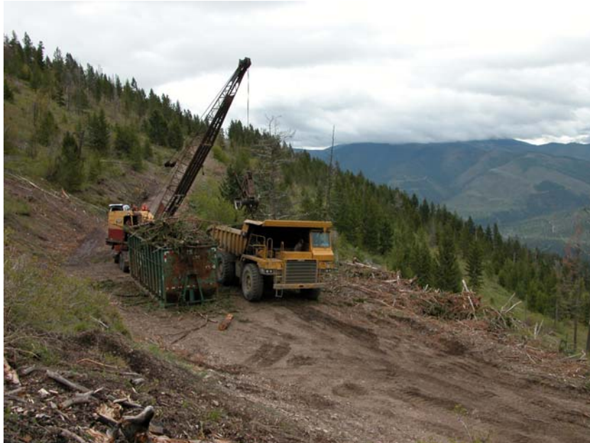
Figure 10. Loading the off-highway dump truck and roll on/off container at roadside landing.
