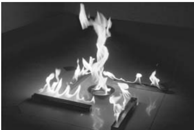
Fig. 4 --Image of fire whirl generated by flow over randomly oriented heat sources.
