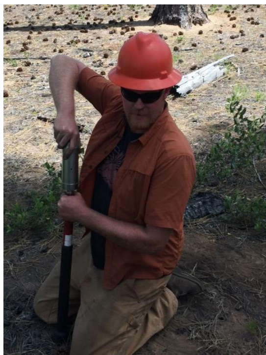
Figure 5 Ben Hart with slide hammer soil corer.
