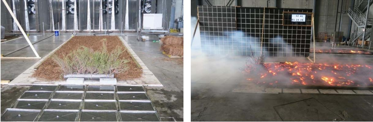
Figure 4. Firebrand Production Experiment - chamise
