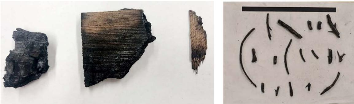
Figure 6. Images Showing Firebrands from Structural (left) and Vegetative (right) Fuels
