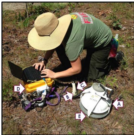
**Figure 4.** Using the LICOR Biosciences LI-8100a (LI-COR Inc, Lincoln, NE, USA), just before the prescribed burn in the OSBS frequently burned unit. Components of the device include: (A) 20-cm soil survey chamber, (B) Omega 8831 type-E soil temperature probe, (C) Decagon Systems EC-5 soil moisture probe (behind temperature probe), (D) LI-8100a device, and (E) 20-cm PVC soil collar.
