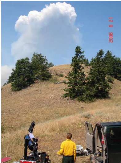
Fig. 3. A smoke plume monitored by the FSL lidar at Tripod Complex Fire (Okanogan, WA) on 21 August 2006. The mean height of the top of the smoke was 7416 m and the maximum fixed height was 8165 m AGL.
