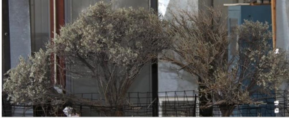
Figure 7. Sagebrush samples placed in the wind tunnel. Wind is from right to left. Horizontal scale is about 2 meters.
