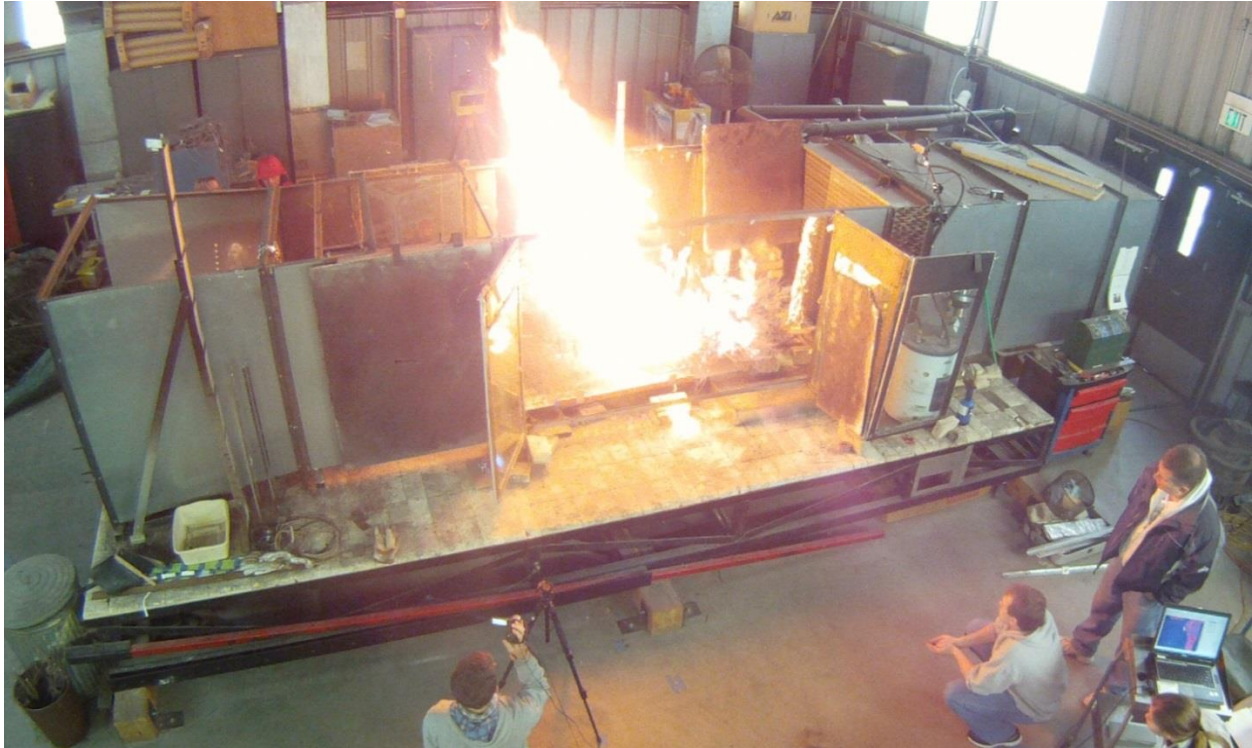
Figure 2. Shrub combustion experiment (chamise) in Riverside Fire Lab wind tunnel. Flaming area is approximately 2 meters long
