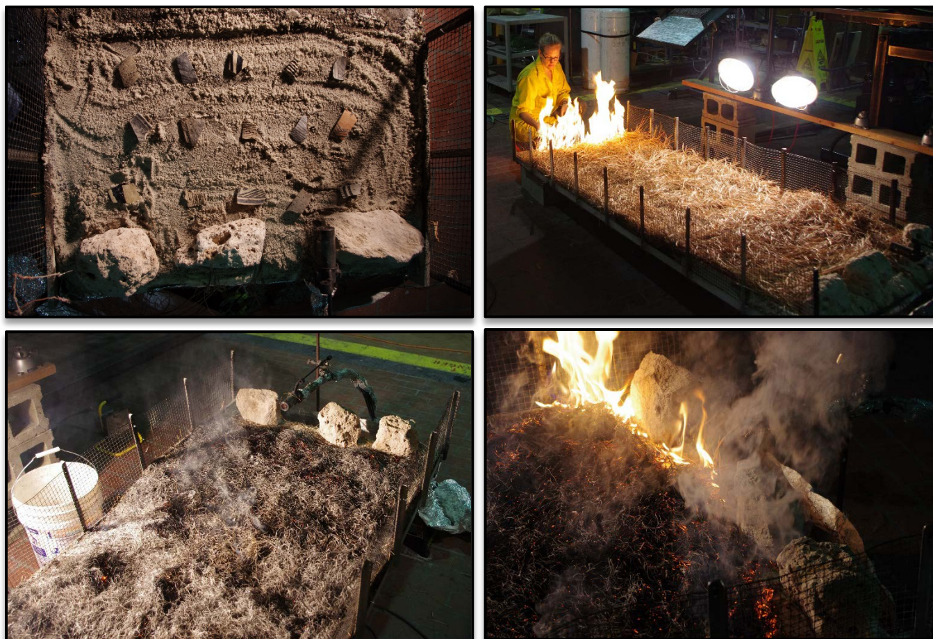
Figure 3. Simulated surface fire environment. Ceramics and masonry on sand bed before fuels and thermocouples are in place (top left); Surface fire bed, ignition (top right); Surface fire bed, after flaming front (bottom left); Flames incident on masonry samples (bottom right).
