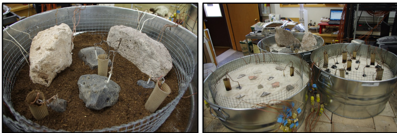
Figure 4. Simulated ground fire environment. Masonry with thermocouples in place, on duff bed (left); Obsidian, ceramics, and masonry with thermocouples in place, before fuels are in place (right).
