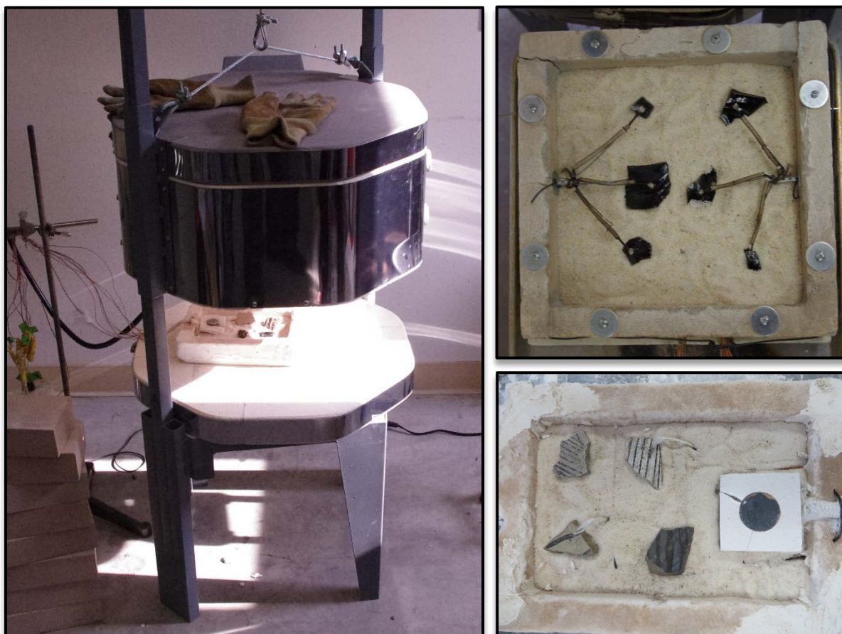
Figure 2. Simulated crown fire environment. Olympic raku kiln with a top hat design (left); Obsidian flakes with thermocouples in place (top right); Ceramics with thermocouples in place (bottom right)
