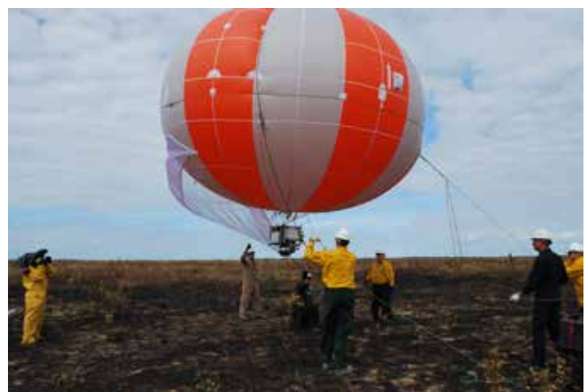
Brian Gullett and the team from the Environmental Protection Agency prepare to launch a balloon into the smoke plume to measure emissions from the forested research burn block.
