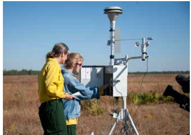
Tara Strand and Susan O'Neal check over an electronic beta attenuation monitor, an instrument for measuring smoke concentrations downwind from the research burns.
