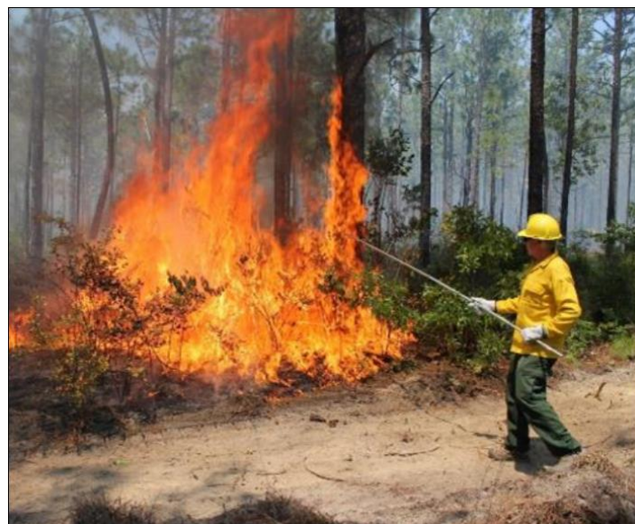
Figure 7 - Rigid tubing (“fishing pole”) used to sample pyrolysis gases produced by heated sparkleberry during May 2017 trial deployment at Ft. Jackson, South Carolina, USA.
